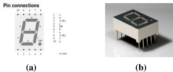
Gambar (a) pin connection ; (b) tampilan fisik seven segment
